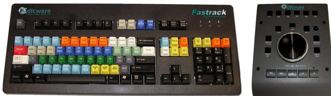
Your Fastrack editing system includes the **K7 Keyboard** and **J6 Jogger Panel**. These devices help streamline work by having most functions available at the press of a key.
