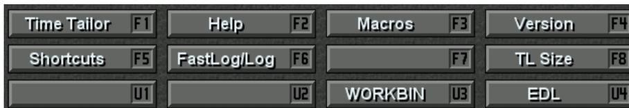
The **Soft Function Keys** correspond to the [F1] - [F8] keys on the K7 Keyboard. The functions displayed on the F-Keys differ depending on which dialog is currently open.
