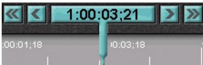
The blue indicator above the Tracks is the **Current Time Indicator**, or **CTI**. The CTI defines the current Timeline location. The arrows next to the CTI are used to jump the CTI around the Timeline.
